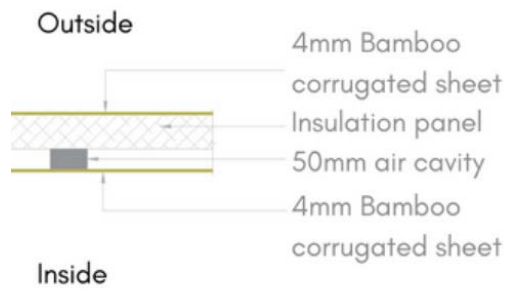
Fig.4 :Flooring composition (Source : Page 24, Team EKAGRA design report)
