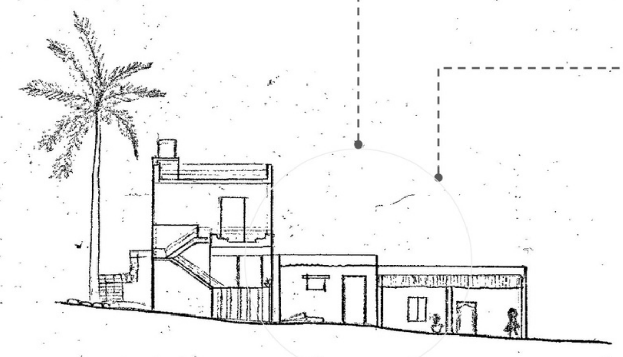
ELEVATION 4D: THIS ELEVATION SHOWS THE PAKKA AND SEMI PAKKA HOUSES WITH DIFFERENCES IN HEIGHTS.
