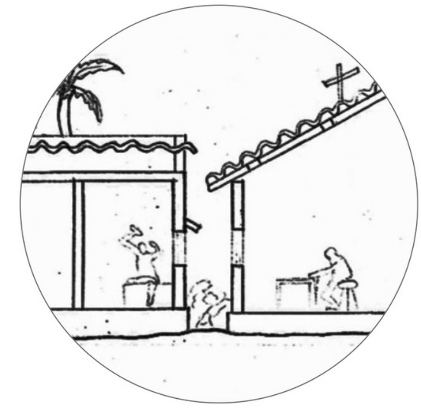
ASBESTOS SHEET AND MANGALORE TILES ARE THE MOST COMMON MATERIAL USED FOR ROOF
