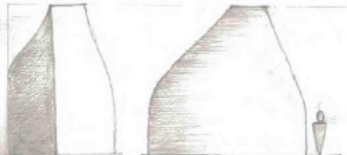
ONE WALL WRAPPED AROUND ITSELF TO FORM A CONE. MADE USING WASTE-EDGED BRICKS OVER A TIMBER FRAMEWORK.
