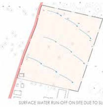
SURFACE WATER RUN-OFF ON SITE DUE TO SLOPE
